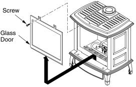
Figure 53 - Removing Glass Door from Burner System
